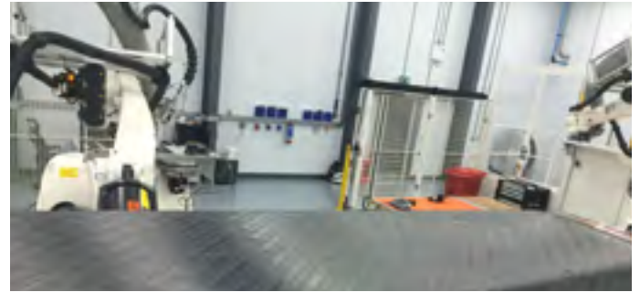
AW169 tail boom upper skin manufactured with laser equipped AFP
