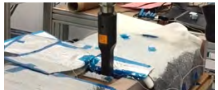
Automated ultra-sonic end effector inserting z-pin (TTR) in composite laminate
