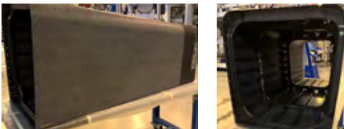
AW169 thermoplastic tail boom demonstrator section
